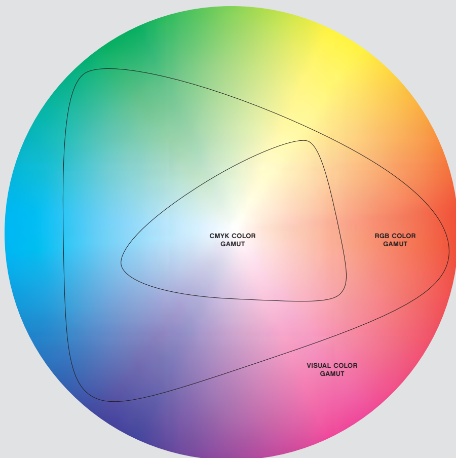
THE SUBTRACTIVE PRIMARIES: CYAN, MAGENTA, YELLOW AND BLACK. IN OFFSET PRINTING BLACK IS ADDED FOR DEPTH, CONTRAST AND RICHNESS OF COLOR
