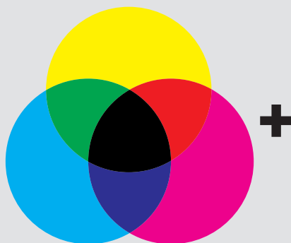
THE SUBTRACTIVE PRIMARIES: CYAN, MAGENTA, YELLOW AND BLACK. IN OFFSET PRINTING BLACK IS ADDED FOR DEPTH, CONTRAST AND RICHNESS OF COLOR
