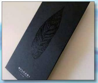
The tricky part when designing a project is the position of the foiled elements in your artwork – particularly if you want the piece to run in one pass on the press. Since each roll of foil physically takes up a certain width, multiple press passes maybe required if the design elements overlap or are very close together. Your printer can help you in the preplanning of your design.
